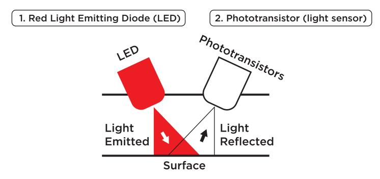
The LED shines light on the surface its driving on and reflects that light into the phototransistor. Try lifting up the robot slightly and have a closer look at the LED light it produces on the surface. Compare how bright the spot of light is when placed on a white surface vs a black surface.
