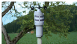
Anemometer - tool used to measure wind speed and direction
