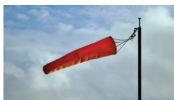
Wind sock - basic tool for measuring wind speed and direction
